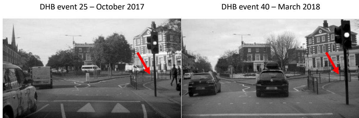
Figure 13 - DHB sequences 25 and 40. Still frames extracted seconds before the harsh braking manoeuvre to demonstrate the obstructed driver view of the upcoming pedestrian crossing (arrow).
