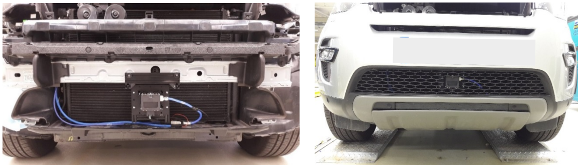
Figure 2 - Hardware adaptations for integration of front radar
