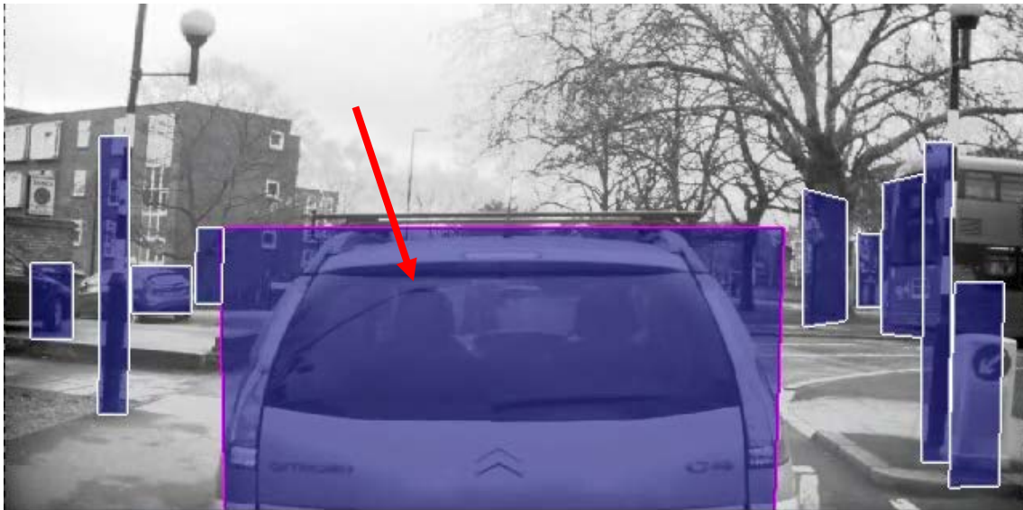
Figure 10 - Leading vehicle triggering Subcritical AEB Sequence 32 in March 2018. Still frame of the trigger extracted from the stereo video recording with boxes indicating camera-detected objects. Red arrow highlights the object causing the trigger.
