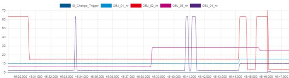
Figure 45 - A view from SFDE showing the change in CAN signals over time for Cut-In candidate 2
