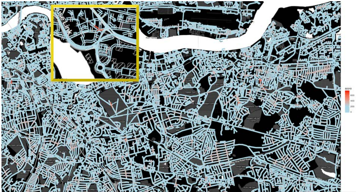
Figure 57 - Risk arising from use of forward-facing sensors with restricted field-of-view, mapped onto Greenwich and surrounding areas. Roads found to be of higher risk appear more red.
