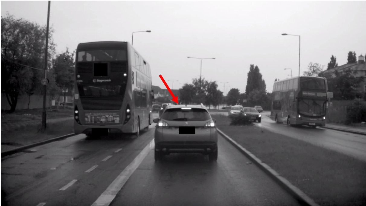
Figure 35 - Leading vehicle triggering Subcritical ARB Sequence 48 in May 2018. Still frame of the trigger extracted from the stereo video recording. Red arrow highlights the object causing the trigger.
