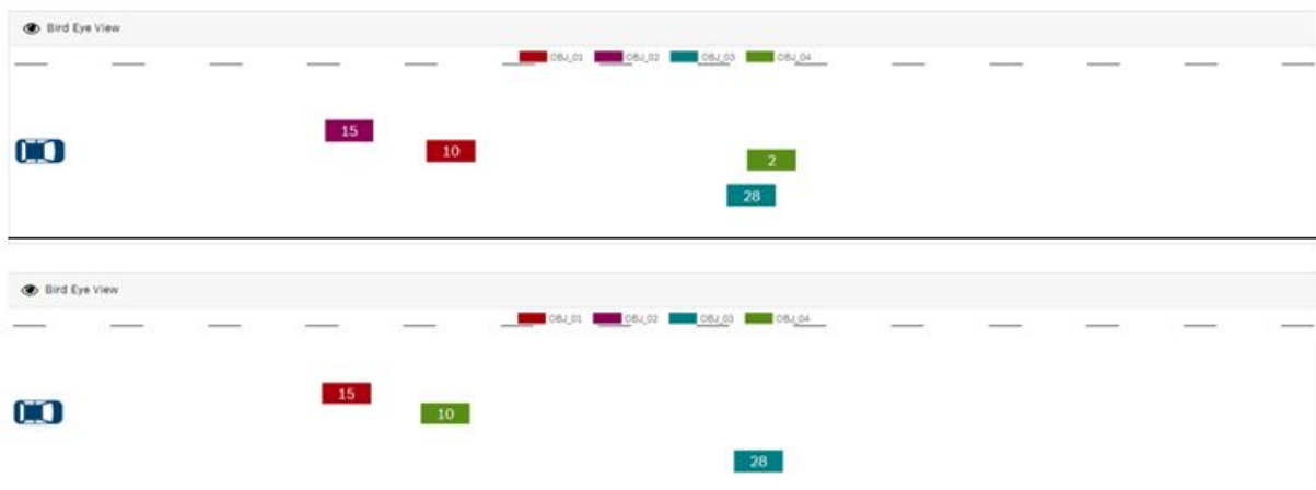
Figure 44 - SFDE bird’s eye view of Cut-In candidate 2 before and after the cut in has taken place
